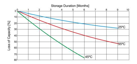
Self Discharge Characteristics @ Different Temperature
